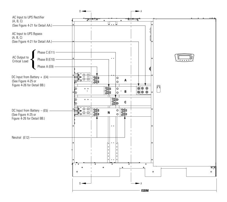
Figure 4-20. ISBM Section Power Terminal Locations – Common Rectifier Feed
